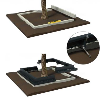
2. Place the two-piece frame on the concrete tires. Bolt the frames with the supplied materials.
